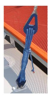
Now to clean up the lashing, just wrap the excess line around the parallel lines, continuing up the lashing. Then tuck the lashing under itself 2 or 3 times to secure it.
