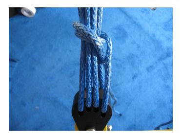
4. Now wrap the line around all of the lashing lines again, taking care to place the line on top of the other wrapped line.
