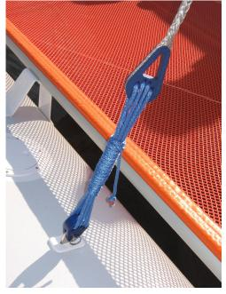
Example of a cleanly tied off shroud lashing on LeeLoo, a Farrier F32RX owned by Mike Seacrest and built by Lombardi Yachts.
