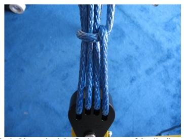
2. Setup the lashing to lead the final output out of the distributor parallel to the other lines.
